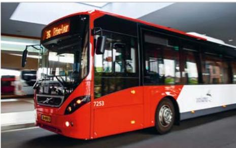
In the Netherlands, DB Arriva put 84 new diesel buses from manufacturer Volvo into service in December 2014 for the transport contract in Brabant. These 13-meter-long buses comply with the Euro VI emissions standard and are suitable both for urban transport and overland transport on medium-range lines. One of the buses is designed for a maximum speed of 100 km/h, for which it was additionally fitted with seat belts.
