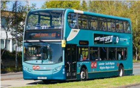
174 additional double-decker buses in the Enviro400 series have been on the roads of Great Britain for DB Arriva since 2015. The first buses were deployed in the North-West region. All are equipped with free WiFi access and CCTV. Using a six-cylinder Cummins-EEV engine, the Enviro400 emits so little carbon dioxide that it meets the Euro VI standard. 48 of these buses were fitted out in superior style for use under the premium brand Sapphire.
