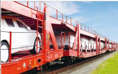
The double-deck wagons of the Laaers 560.1 series are used in the international transport of cars, off-road vehicles and vans. The high load capacity enables particularly heavy vehicles to be transported. The design offers a high degree of flexibility during transport due to fully variable adjustment of the upper loading deck. Mixed loads are thus also possible, in addition to sorted transport. In 2015 the fleet was expanded by adding 113 Laaers 560 to 778.
