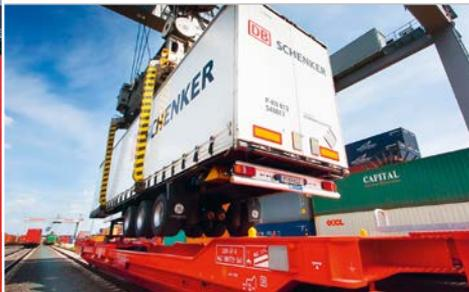
In 2015, DB Cargo acquired a further 259 cars of the Sdggmrs 738.1 series. The double-pocket cars can be loaded with semi-trailers, swap bodies and containers. In comparison with the predecessor to the Sdggmrs 738 series, wear and tear on wheel sets and brake shoes has been reduced even further. This ensures that the vehicles can be operated more cost-effectively.
