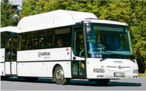
In 2015, DB Arriva bought 32 low-floor buses for use in the Czech region of Moravia. In addition to the 42 seats, 55 standing places increase the capacity of the 12-meter-long bus. Operated with natural gas, the SOR CNG 12 complies with the Euro VI emissions standard. Natural gas engines are quieter than diesel. As an alternative drive technology they are also regarded as particularly eco-friendly. The natural gas tank is on the roof of the bus.
