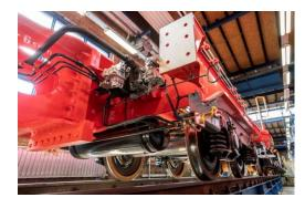
structure of the wagon are flexible, as well as its intended use, for which a length of between 10.8 and 22.6 metres can be selected. The wagon can be quickly converted and reconfigured.
